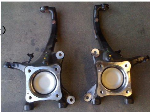
Redesigned Part (Nodular casting iron)
