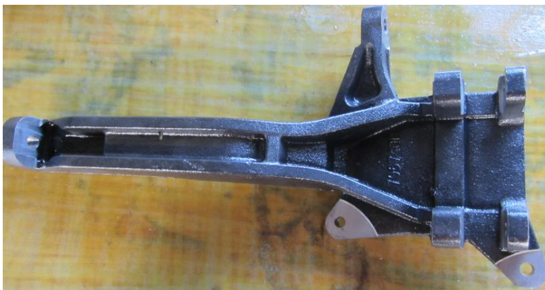
Redesigned Part (Nodular casting iron)
